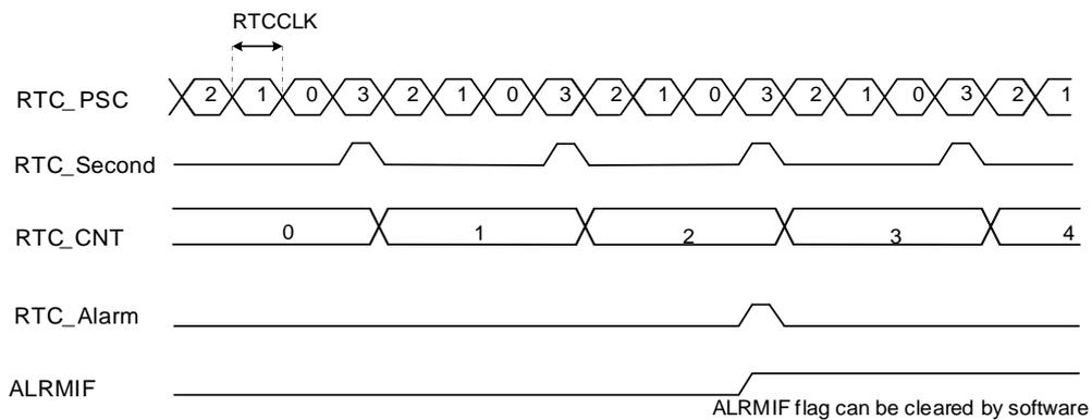
图 14-3. RTC 秒信号及溢出信号的波形(RTC\_PSC = 3)
